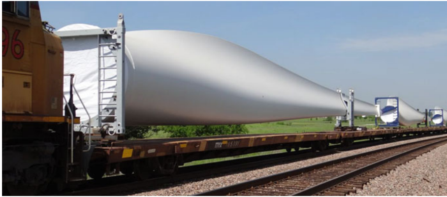
Fig. 11 Rail transport of 55 m blades using custom railcars
