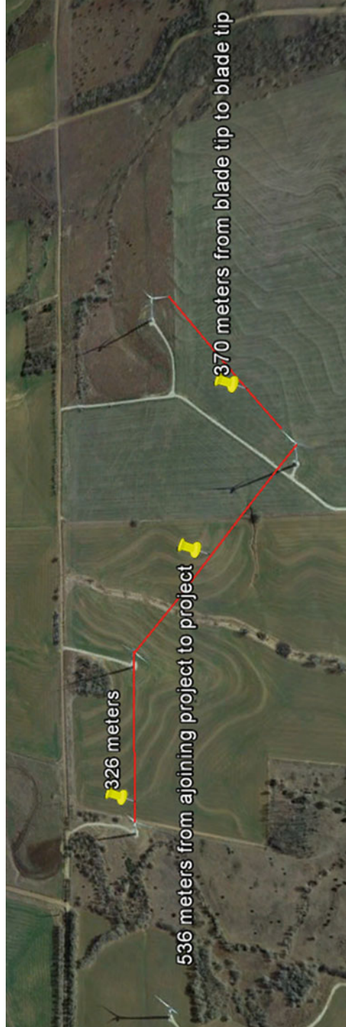
Fig. 5 Microlayout of individual wind turbines Flat Ridge complex KS
