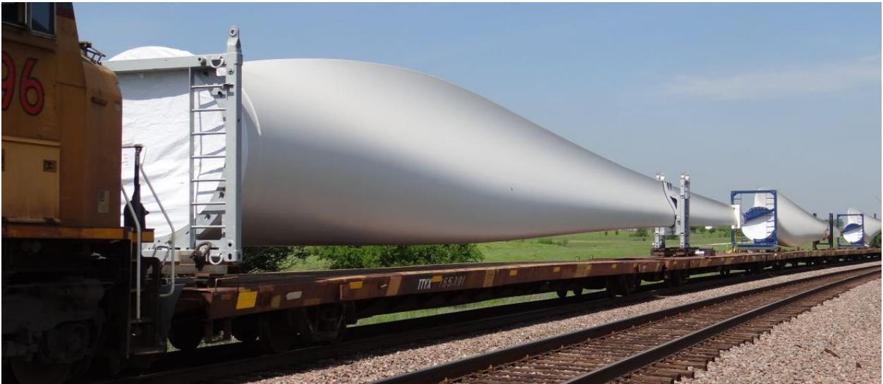
Figure 11: Rail transport of 55 meter blades using custom rail cars
