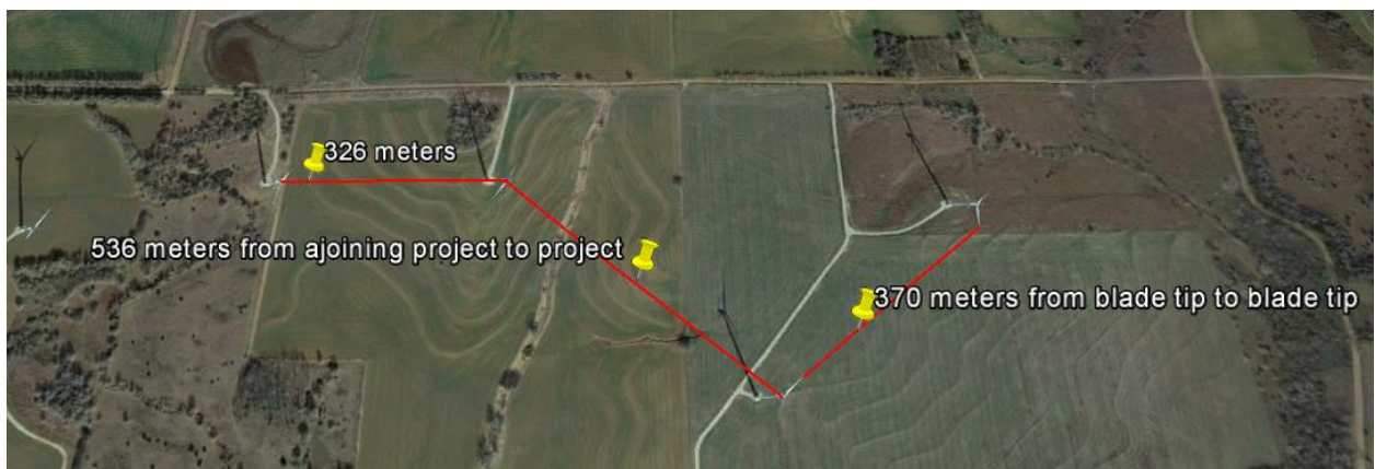
Figure 5: Micro-layout of Individual Wind Turbines Flat Ridge Complex KS
