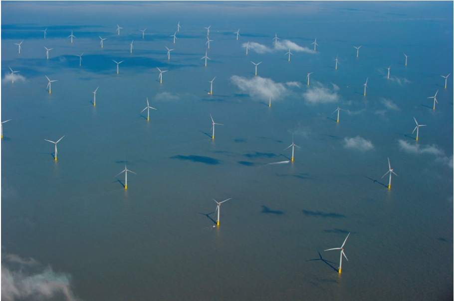
Fig. 4. Aerial view of 20% of the London Array. Here we see 5 legs each with 9 turbines along their length.
