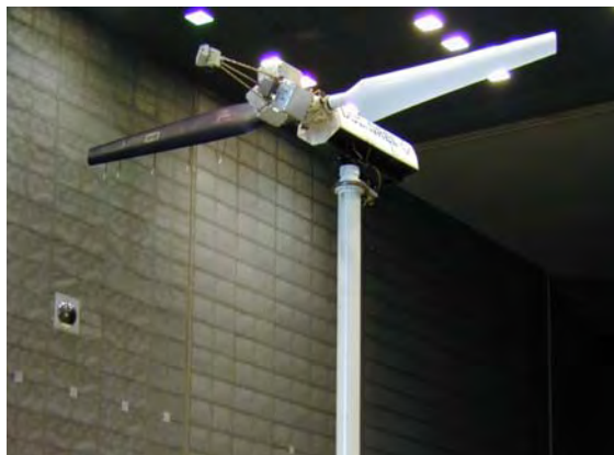
Figure 2: Wind-tunnel testing achieves inflow control, but constrains turbine size.
