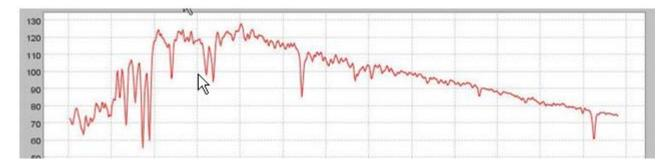
Following a step by step procedure, the end result produced by the user is shown below for measuring the strength of the H-beta line at 4861 Angstroms in this star. The numbers in the two upper boxes represent the wavelength limits of the identified feature and the number in the lower
