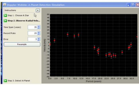
detect a planetary mass and a distance of that mass from the star. The image above represents simulated data for a one solar mass star that has been observed 20 times, over a 35 year period with a radial velocity accuracy of +/- 3 km/s. In the image below, the user employs the fitter and adjusts the mass and distance of the perturbing planet (for comparison the Jupiter-Sun system is shown)
