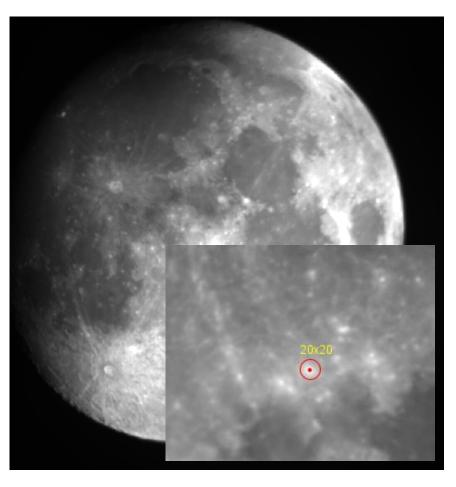
size of lunar Maria and the like). The inset in the picture to the right reveals a small region of the lunar terrain in which a circular aperture of diameter 20 pixels (about 75 km) is overlaid. The teacher/student can use this tool (which is adjustable in size) to measure the radius of circular features (e.g. craters). Of course, this measuring tool will work with any image so it's not restricted to just lunar surface measurements. The second tool involves measuring differences in lunar
