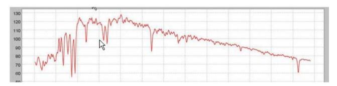
Following a step by step procedure, the end result produced by the user is shown below. The numbers I the two upper boxes represent the wavelength limits of the identified feature and the number in the lower box is the "answer" or the equivalent width of the feature. Again, using this data analysis interface on real stellar spectra is allowing the user to quantitatively measure the strength of a spectral feature using **the same methodology of the real scientist.**
